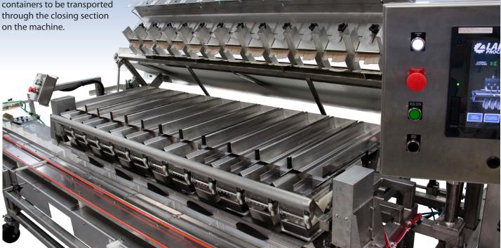
^ Tilt belt and feeder trays easily flip up for guick access and cleaning
