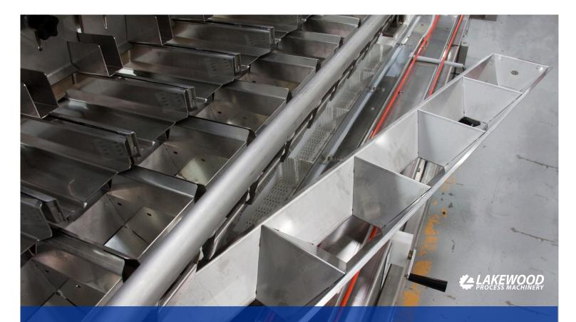
Container changeover is as simple as possible with removable dump funnels for different sized container footprints
