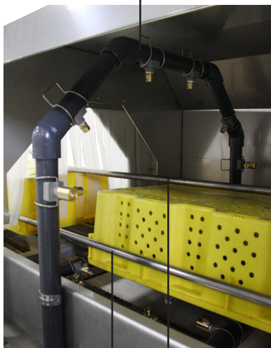
Adjustable Guide Rails Easily adjusted by hand for cleaning different sized lugs
