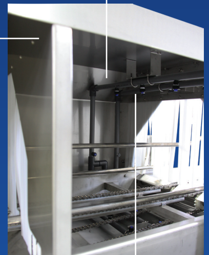
Sanitizing Section (Optional) Includes spray nozzles on all sides
